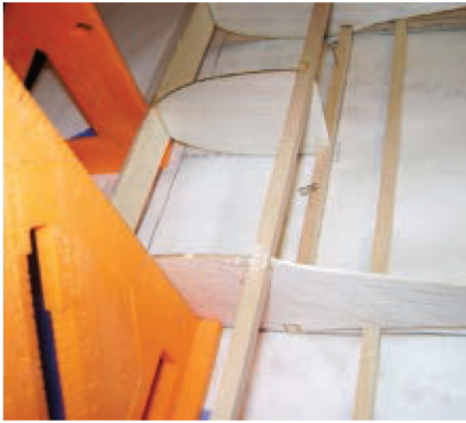
The wing structure is light but strong, and the covering material gives it stiffness. The airfoil is an original reflex Santich design.
